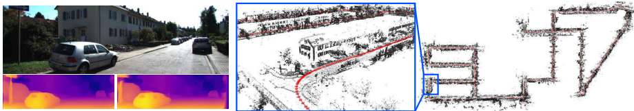
Fig.1: DVSO achieves monocular visual odometry on KITTI on par with state-of-the-art stereo methods. It uses deep-learning based left-right disparity predictions (lower left) for initialization and virtual stereo constraints in an optimization-based direct visual odometry pipeline. This allows for recovering accurate metric estimates.
